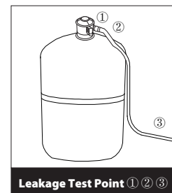
Leakage Test Point ① ② ③
